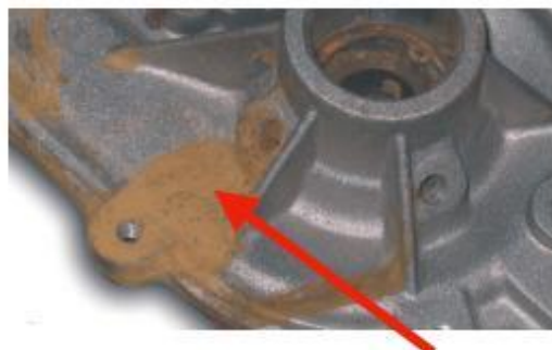
Tell Tale Sign of Water Pump Leak
